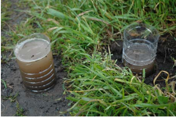
Figure 4. Infiltration tubes in compacted pathway (left), and porous, vegetated soil (right).
